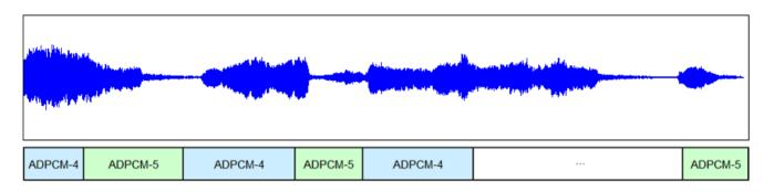
**Solution:** Select the Factor with fixed encoded algorithm, for example, Factor 1 is fixed to 4-bit ADPCM, Factor 9 is fixed to 5-bit ADPCM, or PCM.
